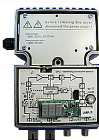
Fig. 5.1. Interior of the MOB-729 optical receiver with a C-729 local monitoring module.
