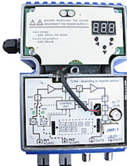
Fig. 5.2. Interior of the MOB-729 optical receiver with a factory fitted M-729 remote monitoring module.
